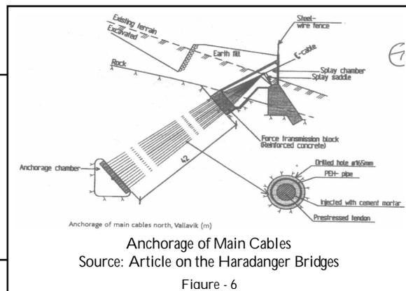
The cable anchorage room of the suspension bridge is one of the most critical elements of design and are suspect to failure as well. Due precautions are taken during the design of the cable anchorage as the fate and longevity of the bridge depend on the quality of anchorage. Also the anchorage with cables at very high tension is prone to corrosion attack.
