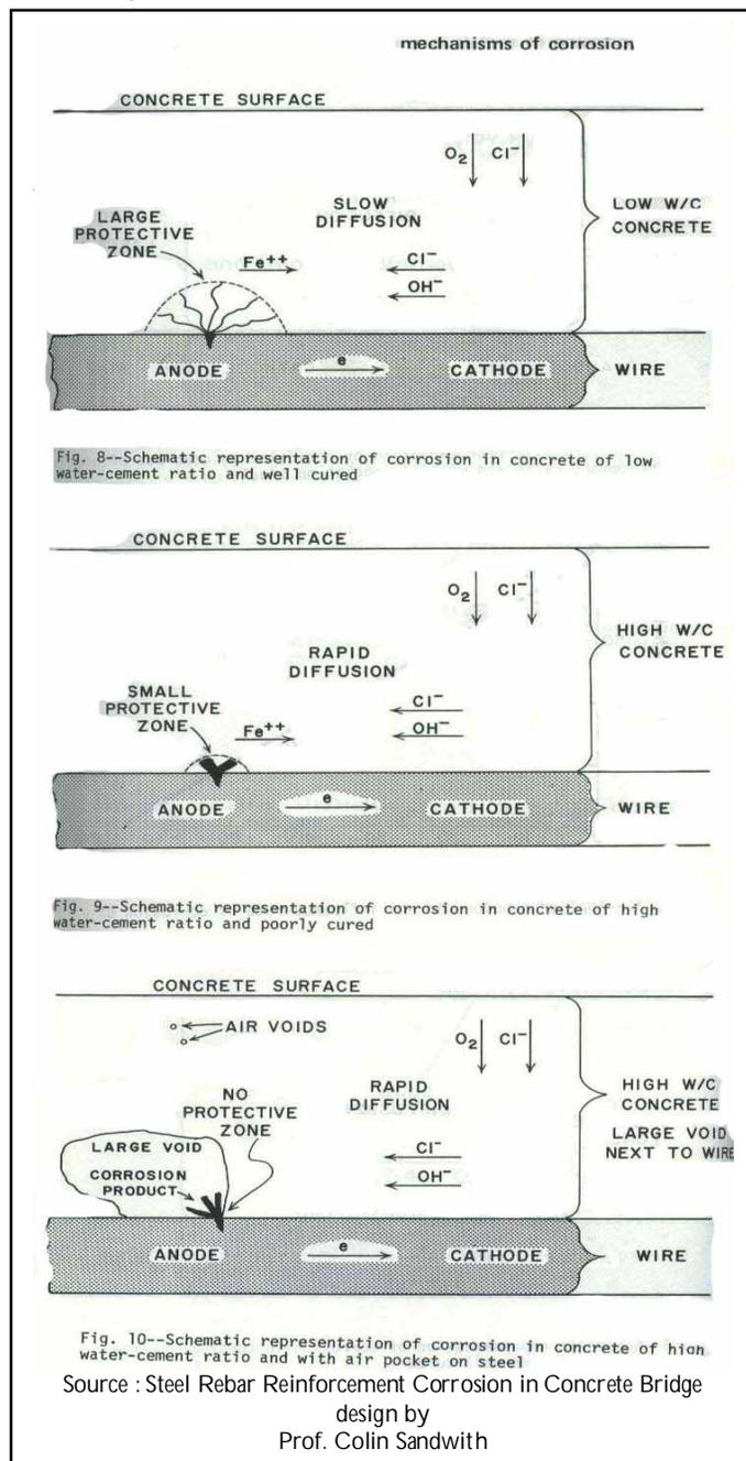
Concrete is a highly alkaline material when first produced (pH range 12-13). The embedded steel is protected by a passive oxide layer, which is maintained by high alkalinity at the surface of the steel.
