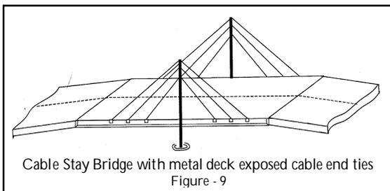
Cable stay bridges have roadways hung from cables. These cables are directly connected to towers. The cable stay can have single metal deck
