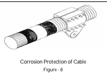
The cables, which are the lifeline of suspension bridges, are protected by dehumidification by wrapping them with loose rubber covers and releasing dry air in the chloroprene rubber jackets. These jackets run over the length of cable maintaining an RH of 40% around them. They are generally applied to the main cables of the suspension bridge:
