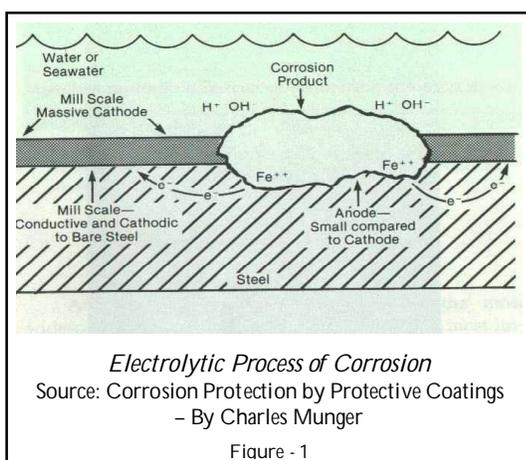
Corrosion is the deterioration of a material, usually a metal that results from a reaction with its environment. Over a period of time the components of a bridge may deteriorate to the extent that the bridge is no longer safe.
