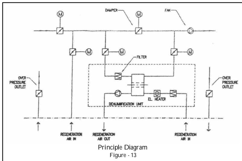
The ventilation fans and the dehumidification units are controlled by 24hrs timer combined with a humidistat and switch in the access doors.
